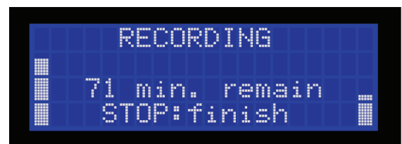
The AIR's screen showing a recording in progress and microphone level indicators
